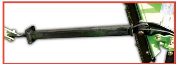
A patented strut arm keeps the arm & mower as one unit. This patented strut arm, in conjunction with the castor wheels, makes movement around signs, bridges and obstacles as easy as a pull of a hydraulic lever. Backing up is a breeze as there is only one pivot point, unlike competitive units.
