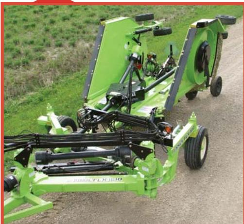
The Schulte FLX-1510 with its new drive system can mow directly behind the tractor as needed with no driveline vibration
